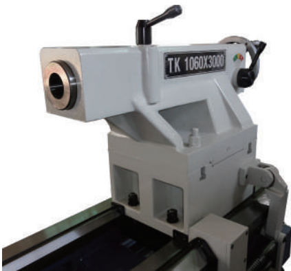
Heavy duty cast iron tailstock body MT6 taper quill movement by 2 speed reduction box and handwheel
