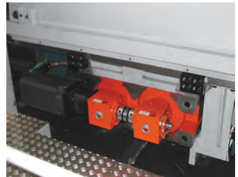
DCMS series machines are precision gear driven when X axis travel is longer than 11M or displacement is faster than 10M/min.
