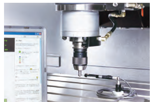
Ball Bar Inspection
