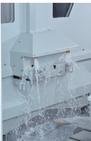
Grundfos chip flush pump greatly enhances APC stability
