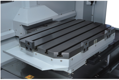
Chip resistant worktable-special internal covers prevent chips dropping into the machine when the APC is in operation
