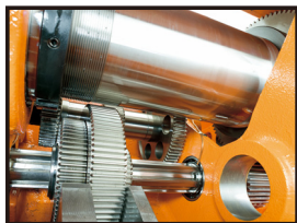
SPECIAL SPINDLE GEAR SET IN HEADSTOCK
