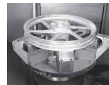
Finger hydraulic chuck
