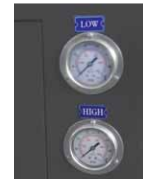
High and low pressure of hydraulic chuck
