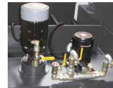
Coolant system (3 bar and more)
