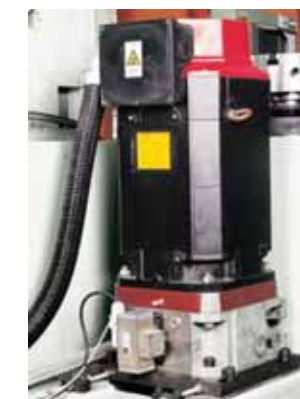
High torque main spindle motor with built-in dual speed gearbox
